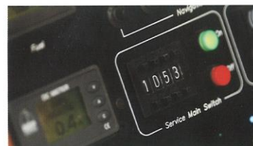
The fuse panel has a code-lock to seal the vessel's main power cutout switch
